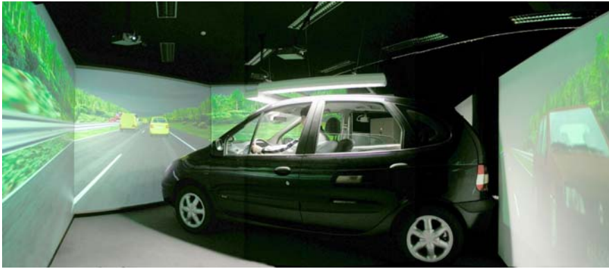
Bild 1: Immersiver Fahrsimulator am Fraunhofer IAO Figure 1: Immersive driving simulator at Fraunhofer IAO Illustration 1: Simulateur de conduite immersif à l'Institut Fraunhofer (IAO)
